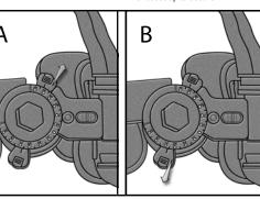
Set Flexion (A) and extension (B) to degrees desired by lifting up tamper pin and slide stop to appropriate degrees. For drop lock, push up slide to lock (C).
