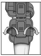
Open strap locks on each of the four sliders with the receiving end of the buckle for size adjustments.
