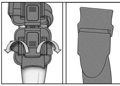
Open strap locks on each of the four sliders with the receiving end of the buckle for size adjustments.
